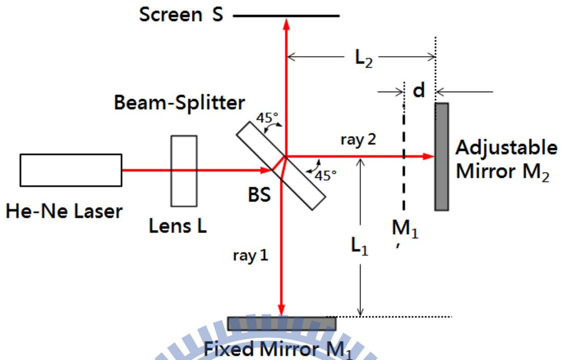
Figure 1. Michelson Interferometer set-up I
