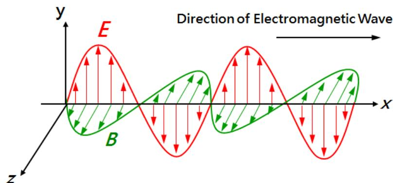
Figure 1. Propagation direction of an electromagnetic wave
