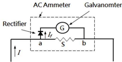
Figure 5. AC Ammeter
