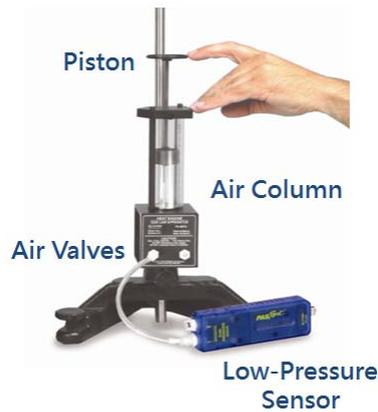
Figure 4. Experiment set-up
