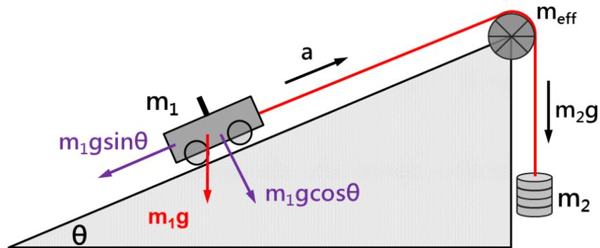
Figure 1. The schematic diagram of the set-up of Atwood's machine experiment
